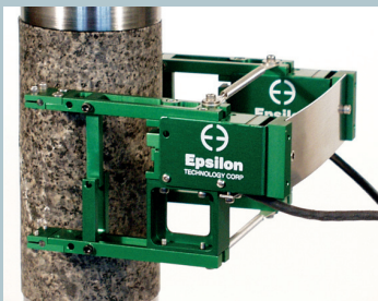
Model 3542RA1 extensometer with 50 mm gauge length
