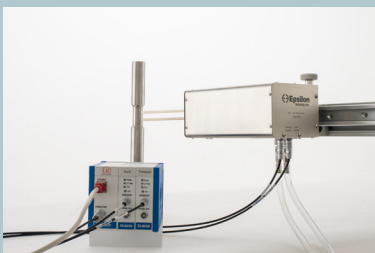
Model 7650 extensometer with Model DT6229 two-channel signal conditioner
